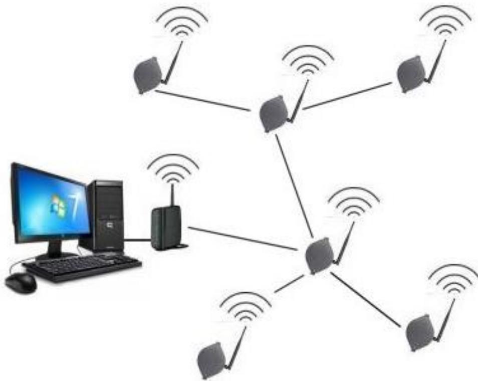
Mesh network transmitter nodes are all able to communicate with each other.
