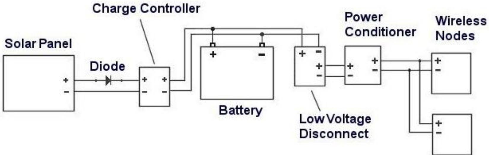
Incorporates a blocking diode you would need to install one.
