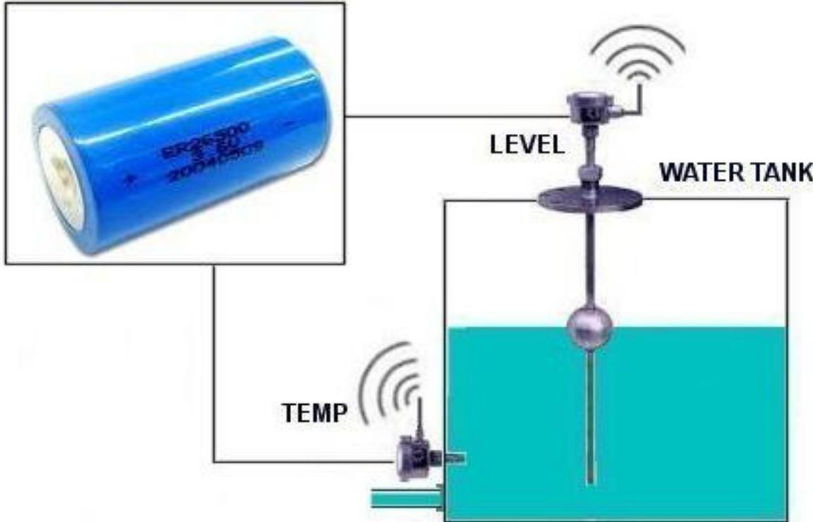
Level and Temperature Transmitter nodes sending data ever 30 seconds (explain cycle-time)
