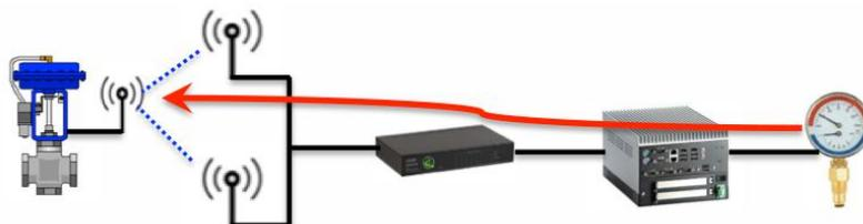
**Figure 5 – Wired sensor, wireless actuator**
