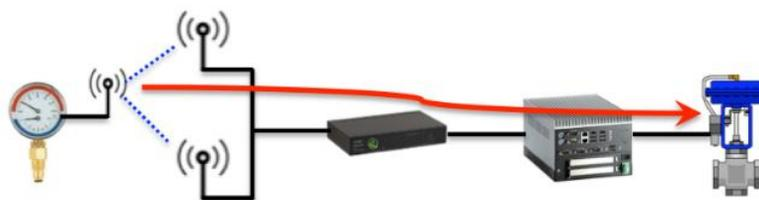
**Figure 4 – Wireless sensor, wired actuator**
